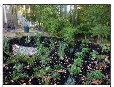
This rain garden infiltrates and filters roof runoff, and has allowed an adjacent eroding area to stabilize.
